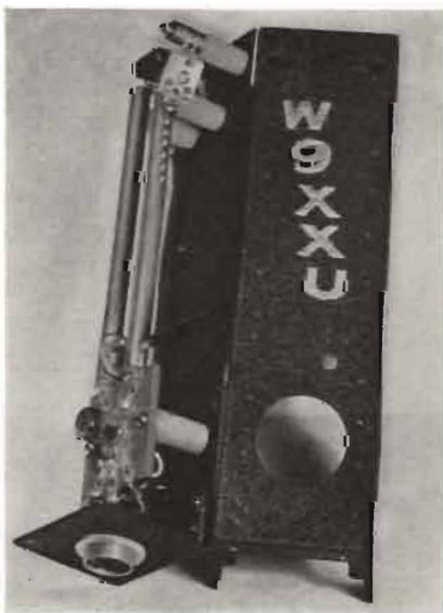
Fig. 5. Side view of 200-mc transmitter. Note \frac{3}{8} " rod tapped for antenna coupling condenser.
