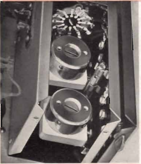
From one to four low-temperature-coefficient quartz plates, housed in a simple temperature control box maintained at 50 deg. C, can be used to monitor any one of four frequencies. The desired channel is selected by a switch on the panel.
