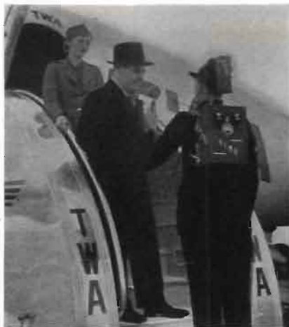
Fig. 2. Showing 300-mc transmitter in use at Kansas City Airport.
