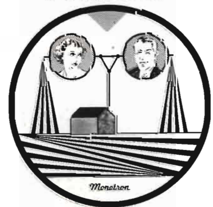
The design printed on metallic disc in the Monotron tube.
