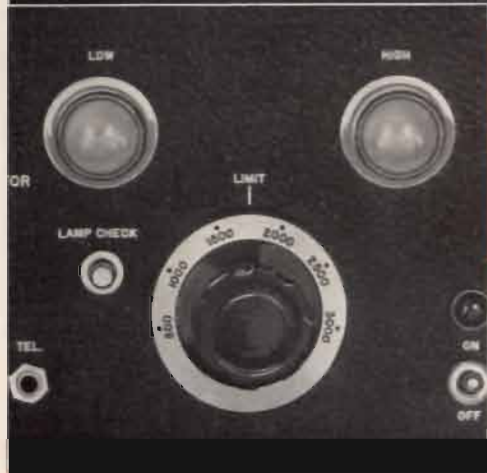
When the transmitter deviates from the assigned frequency by a predetermined amount, one of the warning lamps on the panel lights and indicates direction of deviation.
