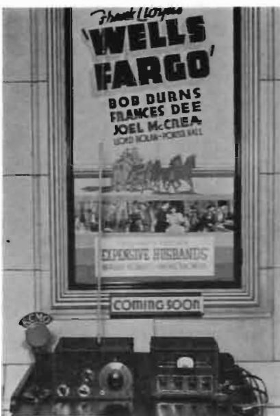
Fig. 6. The receiver and remote amplifier feeding the broadcast equipment.
