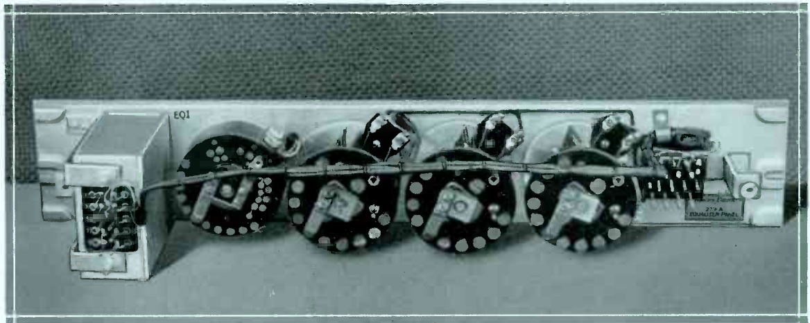
REAR VIEW OF THE 279A EQUALIZER PANEL, COVERS REMOVED. 23A EQUALIZER MOUNTED AT THE LEFT OF PANEL
