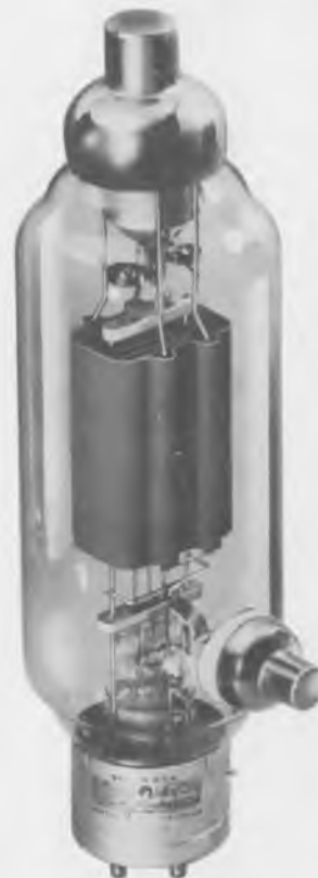
Typical UNITED ELECTRONICS refinements of design are revealed in the above illustration of type KU-23. Individually supported and isolated grid-filament assembly gives this tube the necessary separation between elements for its heavy input ratings. The large anode and wide spacing are design features contributing to the modern efficiency standards which this tube exemplifies.
