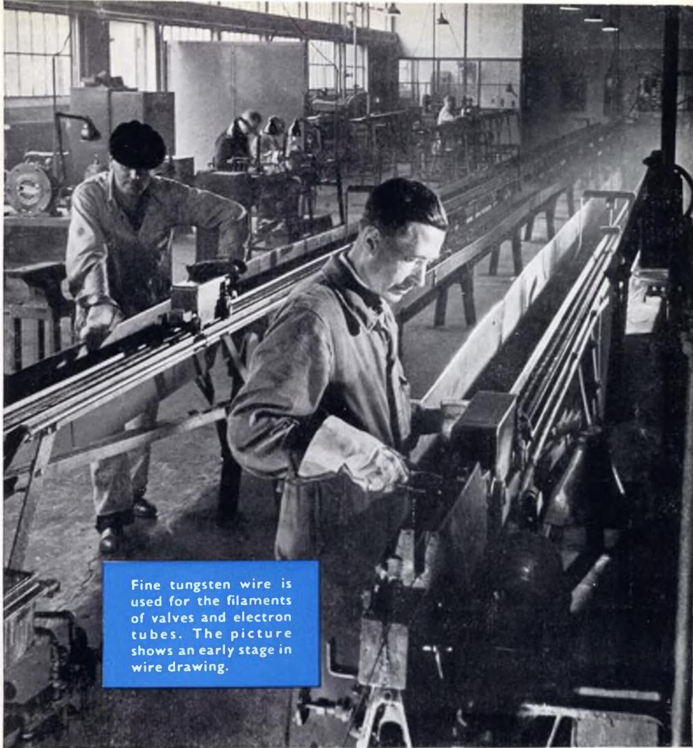
Fine tungsten wire is used for the filaments of valves and electron tubes. The picture shows an early stage in wire drawing.
