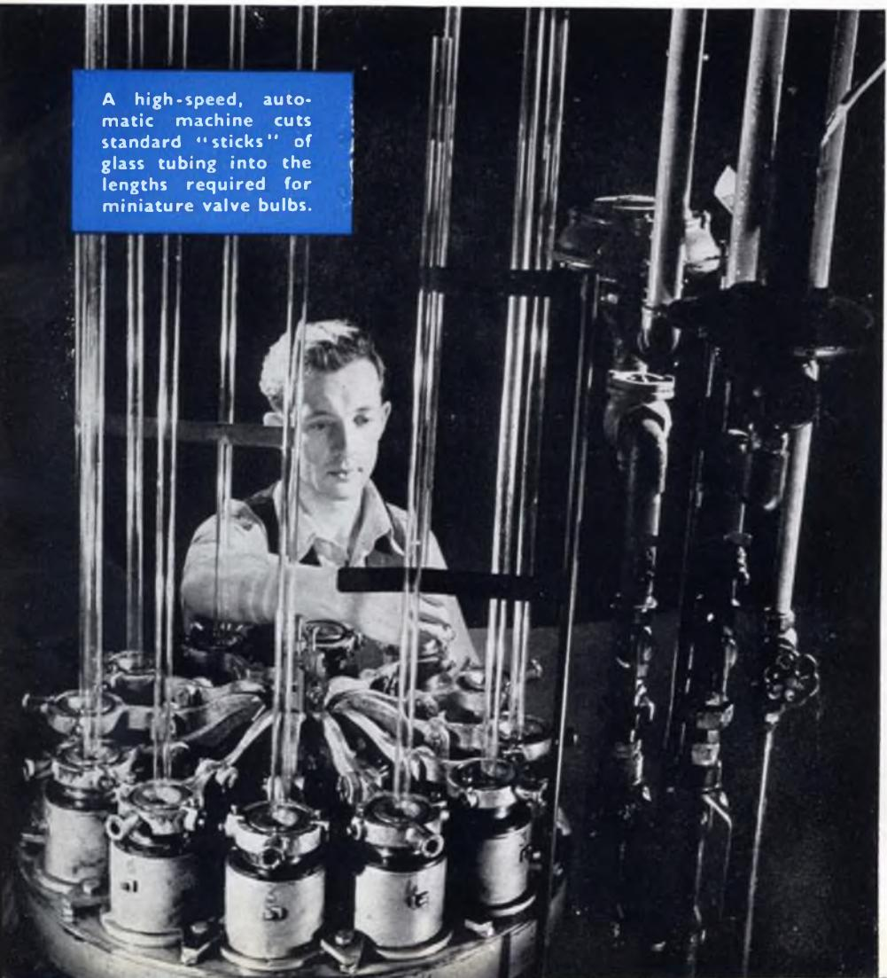
of feet of glass tubing having a wall thickness controlled to tolerances as close as 1/500th inch.
