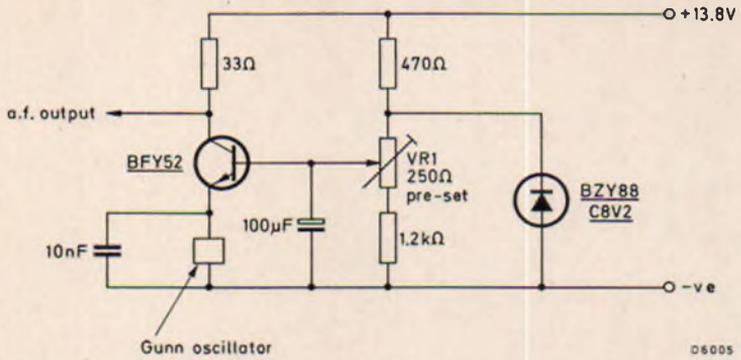
$VR_1$  is used to set voltage at 7.0V across Gunn oscillator.
