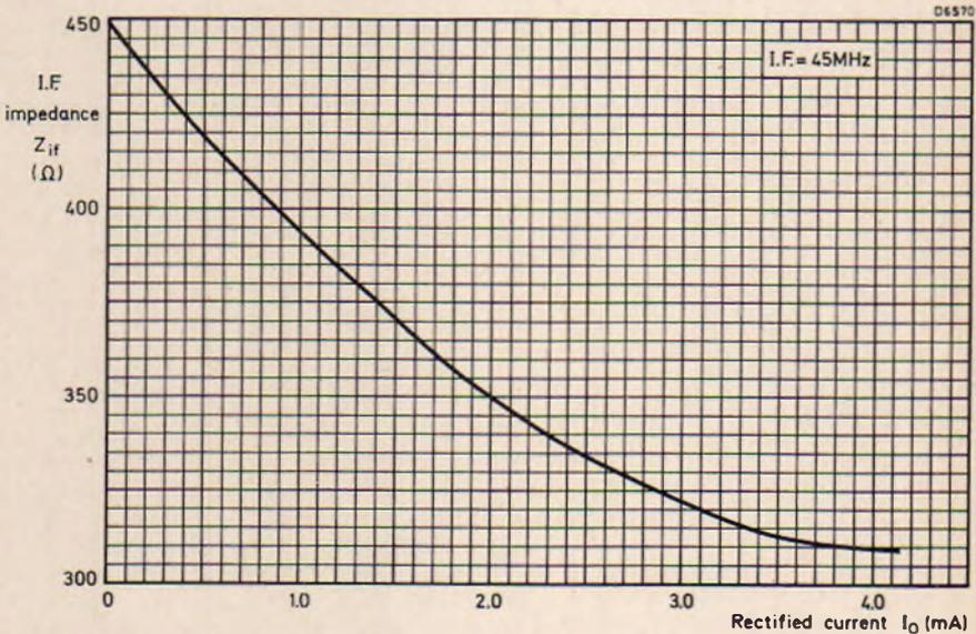
TYPICAL I. F. IMPEDANCE AS A FUNCTION OF RECTIFIED CURRENT
