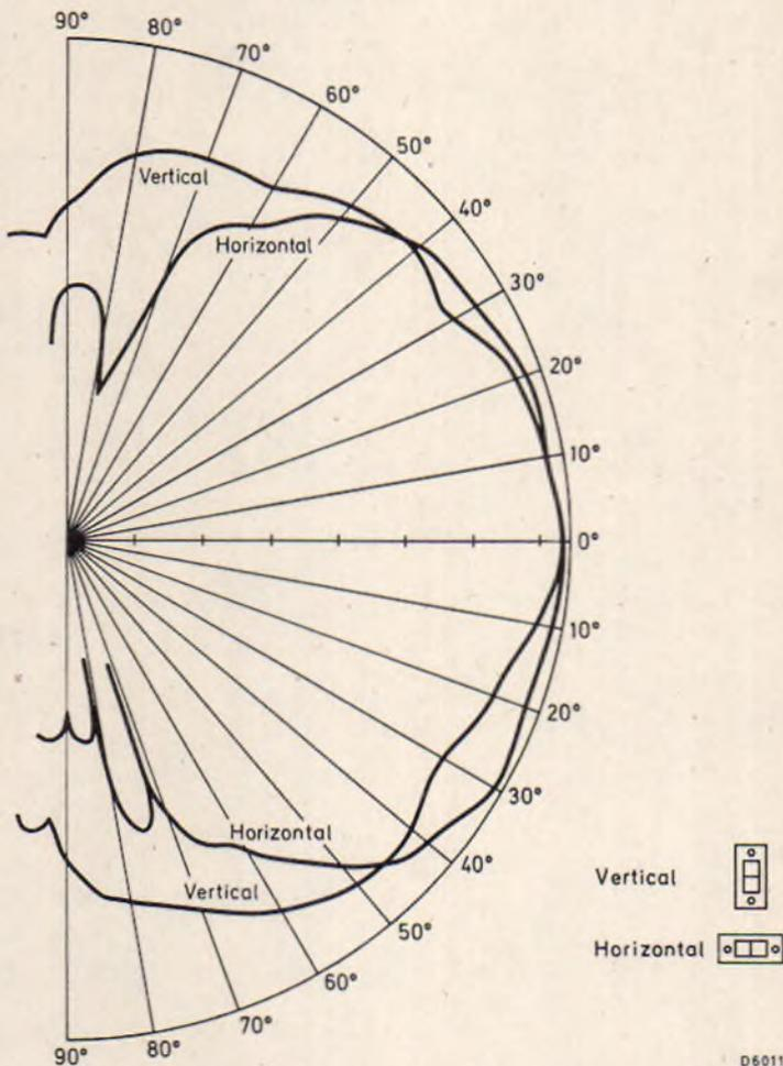
POLAR DIAGRAM FOR ANTENNA SUPPLIED
