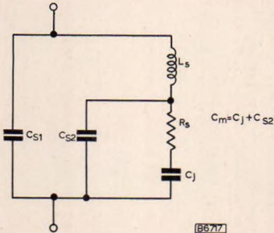
2. Measurements at and about the series resonant frequency, in a suitable waveguide holder, enable the values of  $f_o$  and the diode Q factor to be determined. The effective diode capacitance and the cut-off frequency can be calculated taking  $L_s$  to be the typical value.
