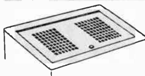
PERFORATIONS IN TOP OF DCR
