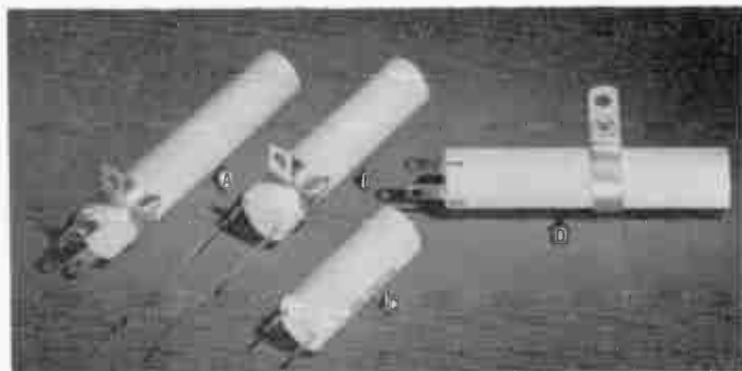
UPRIGHTS A SOLDER LUG TYPE. B PIGTAIL TYPE. C PRINTED CIRCUIT. D HORIZONTAL MOUNTING BRACKET
