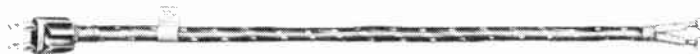
MOLDED VINYL CORD HOLDER PLUG BRAID STRIPPED 1/4" WITH FIBER GLASS TIE, RING TERMINALS FOR #8 SCREW
