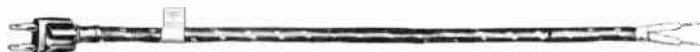
MOLDED VINYL CORD-HOLDER PLUG BRAID STRIPPED 1/4" TIED WITH FIBER GLASS TIE, CONDUCTORS STRIPPED AND TWISTED 3/8"
