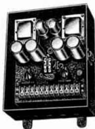
Model 63 Amplifier Door removed to show components.
