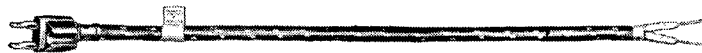
MOLDED VINYL CORD-HOLDER PLUG BRAID STRIPPED 1 1/2", TIED WITH FIBER GLASS TIE, CONDUCTORS STRIPPED AND TWISTED 3/8"
