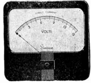
MODELS 29, 39, 49, 59 4 1/2" RECTANGULAR CASE. Width 4 21/32", height, 4 13/64". Mounts in round hole. Body diameter 2 3/4". Scale length 3 29/32". Bakelite case.
