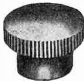
No. 2710—Height 1/2". Diam. 3/4". Metal - faced or plain insert. Female thread available 8-32, 10-32 and 10-24.
