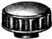
No. 2965 Dia. 7/8". Height from 1/2" to 1 1/4". 1/4" molded hole, metal insert, knurl hole or spring mounting.
