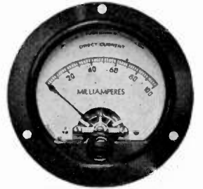
2" ROUND CASE—OPEN FACE STYLE. Flange diameter, 2 3/4"; depth overall, 2 5/8"; body diameter, 2 1/4"; scale length, 1 7/8". Bakelite case.
