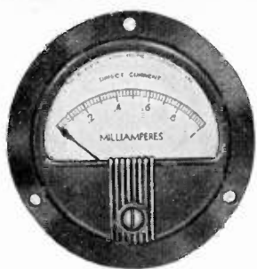
3" ROUND CASE — SHROUD STYLE. Flange diameter, 3 1/2"; depth overall, 2 1/4"; body diameter, 2 3/4"; scale length, 2-9/16". Bakelite case.
