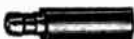
Code S-27 Suppressor—Thread will fit all spark plugs. Most universal type yet devised. Ferrule nut is removable. 5000 ohms.
