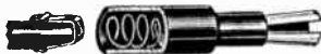
Code T-20 Distributor Suppressor—Cable clip snaps into suppressor. 10,000 ohms. Not necessary to remove clip on cable and therefore suppressor can be quickly removed for ignition testing purposes.
