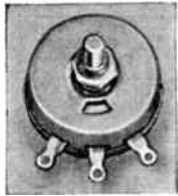
Dissipates 4 Watts — Insulated Contact Arm. Use Dial Plate No. 395. 294° total rotation; 281° effective electrical rotation. Prices include one No. 232 Nut.
