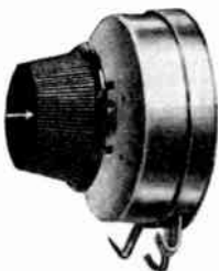
Dissipates 9 Watts—Contact Arm Grounded. Use Dial Plate No. 399. 318° total rotation; 304° effective electrical rotation. Prices include one No. 232 Nut.
