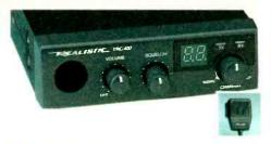
NEW! TRC-437. Electronic channel controls. Squelch and volume control. ANL. LED channel indicator, LED transmit/receive indicators. Remote speaker jack. Only  $1^{1/4} \times 4^{1/4} \times 6^{3/4}$ ". (TSP) **21-1553** ..... **59.95**
