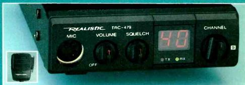
TRC-479. Never drive "alone" again. Our lowest priced mini transceiver mounts easily under dash to provide extra security and convenience on the road. Automatic Noise Limiter (ANL) cuts pulse-type noise. Dual ceramic filters provide
