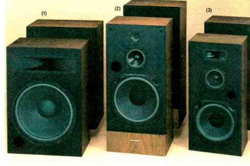
(1) Realistic Nova®-18. An excellent low-priced 2-way system for high-powered digital audio. The tuned-port bass-reflex design and 10" long-throw woofer combine for rock-solid low-frequency response, and the 3" tweeter is ferrofluid-cooled for crisp highs with low distortion. Genuine walnut veneer. Removable cloth grille. Response: 65-20,000 Hz. Power handling capacity: 100 watts. 225/8 × 123/16 × 81/8".
