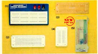
The fast way to design your own circuits! Our breadboards accept a wide variety of devices and make circuit changes as easy as plugging and unplugging wires. When your circuit is working properly, it's simple to transfer it to the matching experimenter's PC board for a soldered, permanent version.
