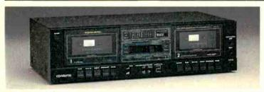
Response: ±3 dB: 60-14,000 Hz (metal), 60-12,500 Hz (CrO<sub>2</sub>/Hi-Bias/Type II), 60-10,000 Hz (normal/Type I). Wow and Flutter: 0.12 % WRMS. S/N: 70 dB Dolby C; 62 dB Dolby B (ref. 3.0% distortion, "A" weighted, metal tape). Distortion: 1.0% 3rd HD. Record/Play Head: Permalloy. Erase Head: Ferrite. Size: 45/16 × 169/16 × 81/4".
