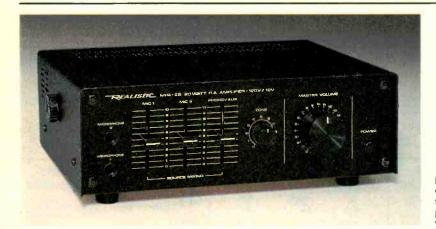
SPECIFICATIONS. Frequency Response: 150-20,000 Hz ±3 dB. Power: 20 watts rms at 8 ohms. Outputs: 4, 8, 16 ohms; 70V line. Power Requirement: 120VAC, 60 Hz, 40W or 12VDC negative ground. Size: 41/2 × 101/2 × 71/2".
