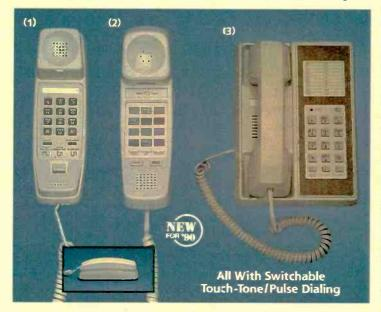
(1) Radio Shack ET-282 Slim-Fone<sup>™</sup>. Auto-dials up to 20 phone numbers of up to 16 digits each. Redial button with pause for systems requiring access code. Hi/ lo/off ringer control.
