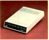
Intelligent Modem DCM 212. Features menu-driven operation that automatically selects 300 or 1200-bps rate. Bell 212A-compatible asynchronous operation. Connects via RJ-11. FCC registered. UL listed AC.
