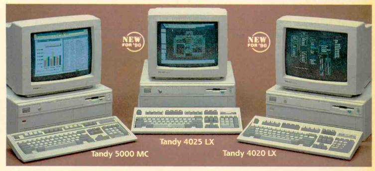
The high-performance answer for power users. IBM<sup>®</sup> Micro Channel<sup>™</sup> compatible archi-tecture provides a fast 32-bit data path. The 5000 MC's Intel® 80386™ microprocessor operates at 20 MHz, and a memory cache controller provides RAM-fast access to your data. 2 MB RAM, VGA graphics built in. UL listed AC. 25-6000\* (TSP available) .... 4999.00
