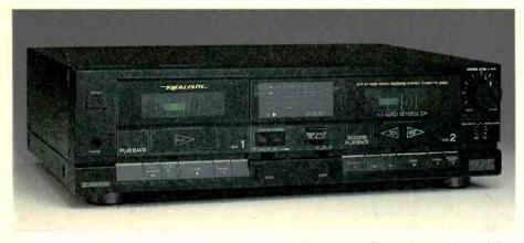
**Response:** ± 3 dB: 20-17,000 Hz (metal), 20-16,000 Hz (CrO<sub>2</sub>/Hi-Bias/Type II), 20-15,000 Hz (normal/Type I). **Wow and Flutter:** 0.06% WRMS. S/N: 70 dB Dolby C; 62 dB Dolby B ("A" weighted, metal tape). **Distortion:** 1.0% 3rd HD. **Record/Play Head:** Permalloy. **Erase Head:** Ferrite. **Size:** 5 × 16<sup>15</sup>/16 × 12<sup>9</sup>/16".
