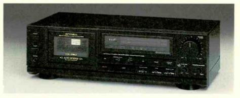
**Response:** ± 3 dB: 20-18,000 Hz (metal), 20-17,000 Hz (CrO<sub>3</sub>/Hi-Bias/Type II), 20-16,000 Hz (normal/Type I). **Wow and Flutter:** 0.065% WRMS. S/N: 78 dB Dolby C; 65 dB Dolby B (metal tape). **Distortion:** 1.0% 3rd HD. **Record/Play Head:** Permalloy. **Erase Head:** Double gap ferrite. **Size:**  $5 \times 17 \times 9^{1/4}$ ".
