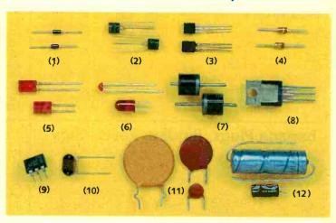
(7) 5 Rectifiers. Rated 6 amps, 50 PIV. 276-1661 ..... 1.98 (8) 5 Voltage Regulators. Includes one 7805, one 7812 and three other types. 276-1660 ..... 1.98 (9) 3 Optocouplers. Three different types. 276-139 ..... 1.98 (10) 5 Photocells. CdS photoresistors. Excellent for experiments. Various styles and ratings. 276-1657 . . 1.98 (11) 100 Disc Capacitors. May include NPO, Hi-Q, N-750, Mylar and ceramics. 272-801 ..... 1.98 (12) 20 Electrolytics. Assorted values and styles. 272-802 ..... 1.98
