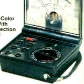
Fuse/surge-absorber protected. Sensitivity: 20,000 ohms per volt DC. Measures to 1200 volts DC in seven ranges, 1200 volts AC in five ranges, DC current to 300 mA in four ranges, resistance to two megohms in four ranges, and decibels - 20 to +63 in five ranges. Accuracy ±3% DC, ±4% AC. Open, 71/4 x 45/16 x 11/4". Requires "AA" battery. 22-211
