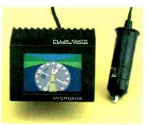
Obsoletes ordinary compasses! High-tech circuitry measures the earth's magnetic field in two directions and compensates for stray magnetic fields, giving you a full-color, illuminated 360° graphic display of your auto's direction. Mounts on dash or windshield. Connects directly to electrical system or plugs into lighter socket with included adapter. 21/8 x 3 x 27/8". 12VDC neg. gnd. 63-641 ...
