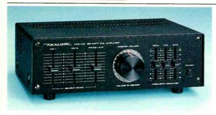
SPECIFICATIONS: Frequency Response: 70-15,000 Hz + 1/-3 dB. Power: 35 watts rms at 8 ohms. Outputs: 4, 8, 16 ohms; 70V line; terminals for adding optional SPST switch for remote priority switching. Power Requirement: 120VAC, 60 Hz, 120W. Size:  $41/2 \times 101/2 \times 71/2^n$ .
