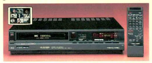
Realistic Model 72. Much more than an ordinary VCR. You get easy on-screen programming, exciting new digital effects and wireless remote control. Strobe mode displays a full-screen still picture that is updated by new stills at fixed or variable intervals.
