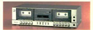
Response: ± 3 dB: 60-14,000 Hz (metal), 60-12,500 Hz (CrO<sub>2</sub>/Hi-Bias), 60-10,000 Hz (normal). Wow and Flutter: 0.12% WRMS. S/N: 70 dB Dolby C: 60 dB Dolby B (ref. 3.0% distortion, "A" weighted, metal tape). Distortion: 1.0% 3rd HD. Record/Play Head: Permalloy. Erase Head: Ferrite. Size: 4% 6 x 16% 6 x 814".
