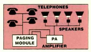
Now you can turn your Touch-Tone telephone into a public address system. This module lets you connect your telephone to a PA amplifier. Once connected, just lift the handset, press " \*" button and talk. If
