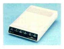
Intelligent Modem DCM 212. Features menu-driven operation that automatically selects 300 or 1200 bps rate. Bell 212A-compatible asynchronous operation. Connects via RJ-11. FCC registered. UL listed AC. 26-1385
