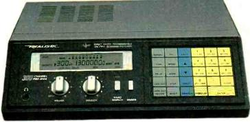
stored in a special, eleventh bank for instant one-key transfer to regular memory. Automatic and manual scanning steps. Two-speed scan and search. Sound-squelch control prevents lockups on unmodulated carriers. All this plus priority mode, scan delay, channel lockout. Jacks: 1/8" headphone, Ve" external speaker, phono-type tape out, BNC antenna input, external DC power. Memory backup requires 9V battery. 213/16 x 1011/16 x 811/16". UL listed AC (or 12VDC cable, extra). 20-119 .... 419.95
