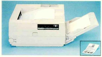
SPECIFICATIONS: Print Speed: 6 pages per minute. Resolution:  $300 \times 300$  dots per inch. Printable area max. 8'' wide,  $13^3/2''$  long. Paper Size: Letter, legal, half-letter, A4, A5, B5, 4 to  $8^1/2''$  wide and  $8^5/_{16}$  to 14'' long. Paper tray holds 150 sheets 20# bond max. Duty Cycle: 3000 sheets per month. Interfaces: Video, Centronics parallel. Dimensions:  $8^5/_{16} \times 16^1/_{16} \times 16^1/_{2}''$ . Weight: 37.5 lbs. Power: 120 VAC, 60 Hz. UL listed AC.
