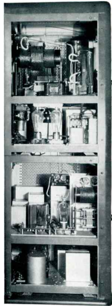
An interior view of the left side of the transmitter. Easy accessibility to all parts featured throughout.
