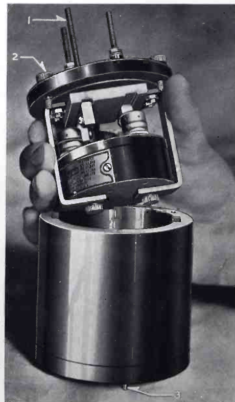
FIG. 2—PLACING CRYSTAL MOUNTING IN WELL
