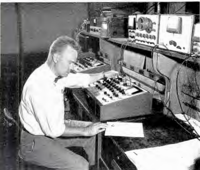
Using MicroMhoMeter to check electron tube performance.
