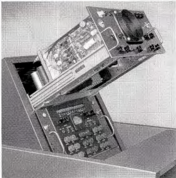
Type TO-1 Oscilloscope mounted with Color Camera Processing Amplifier in standard 22-inch console housing. The oscilloscope is compactly housed on a drawer-type chassis which glides in or out on heavy gauge aluminum slides which lock in the extended position.
