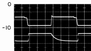
G. Top: Q11 base, 10 \mu\text{s}/\text{cm} , 5\text{v}/\text{cm} Bottom: Q11 collector, 10 \mu\text{s}/\text{cm} , 5\text{v}/\text{cm}
