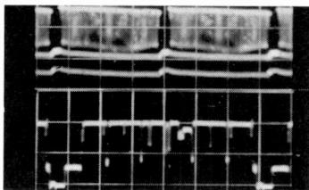
A. TP1 Top: 5 ms/cm, .5v/cm Bottom: 10 μs/cm, .5v/cm
