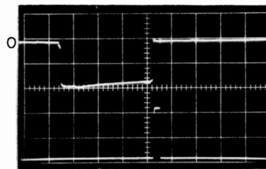
E. Top: Q40 base, 10 μs/cm, 5v/cm. Bottom: Q44 emitter, 10 μs/cm, 2v/cm
