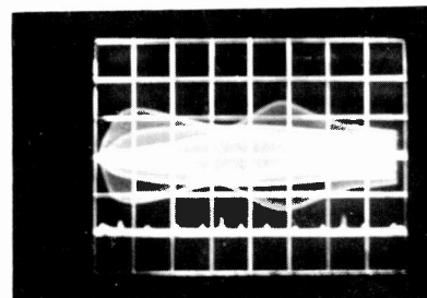
Fig. 53 Composite Waveform Showing Response of Playback Amplifier
