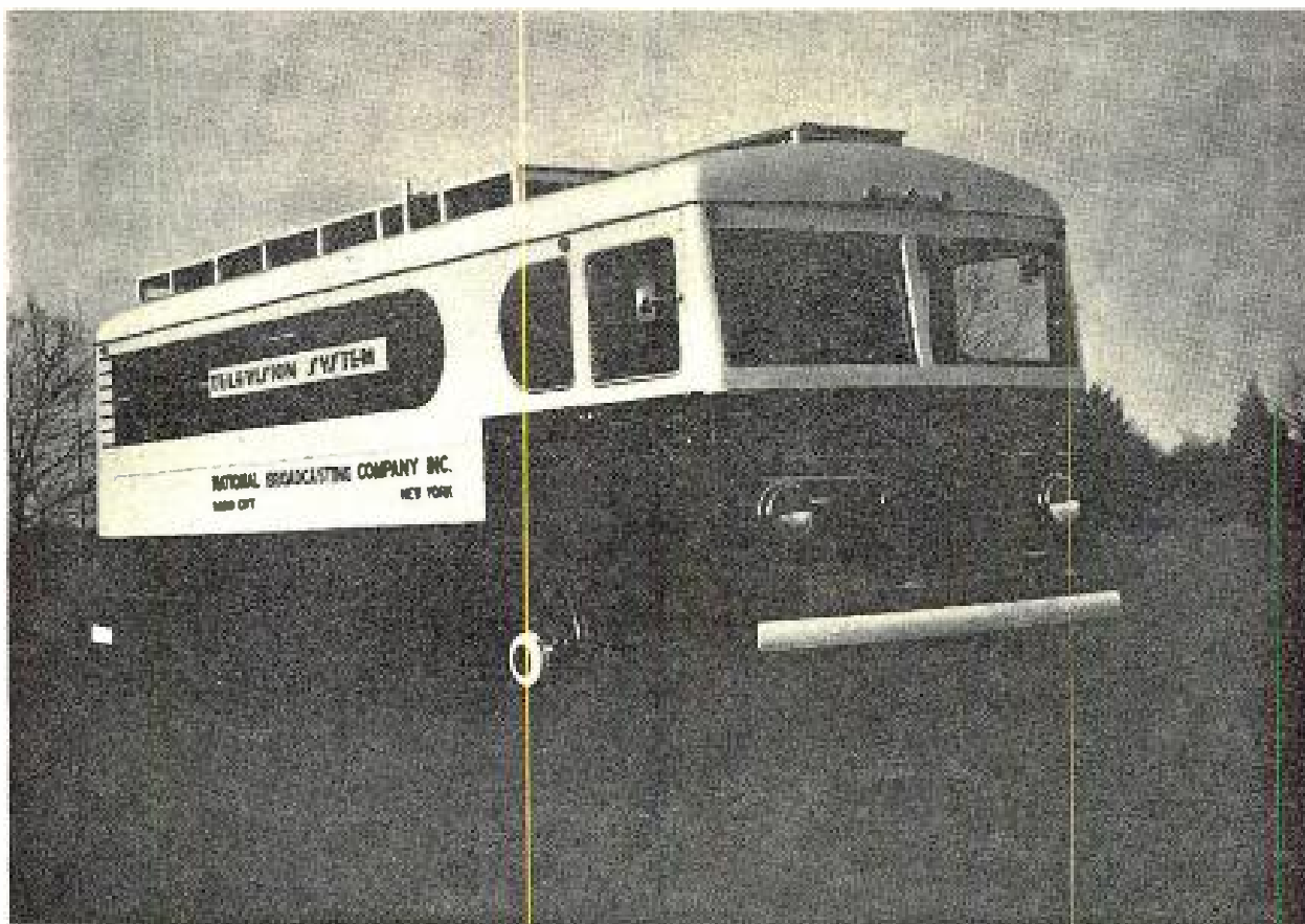
Fig. 6 – Color television mobile unit, 1952.
