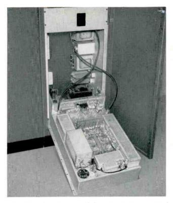
Aural and wisual exciter circuits of the TTL-100AL/AH are mounted on a single hinged chassis allowing access to transformers, filters and other components housed in bottom of transmitter cabinet.
