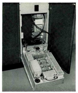
Aural and visual exciter circuits of the TTL-500AL/AH are mounted on a single hinged chassis allowing easy access to all components.
