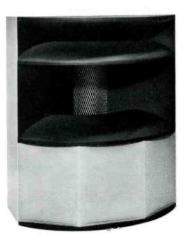
The LC-9 Loudspeaker System is designed for applications where high acoustical level, wide dispersion angle, and extended frequency response are required. The frequency range is covered by separate low and high frequency horns with a crossover point at 500 Hz. A feature of the LC-9 is the particular care with which the high and low frequency horns have been designed to provide matched acoustical wavefronts for smooth response over the entire frequency range.
