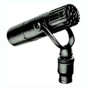
A dependable, high-quality ribbon instrument with an improved cardioid directional characteristic, the RCA Type BK-5 Microphone offers essentially flat frequency response from 30 to 20,000 Hz. Its smooth response and wide frequency range make it ideal for both speech and music.
