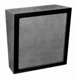
An open-back bafflle for any standard 8- or 12-inch loudspeaker, the MI-11414-2 unit is built of one-half-inch plywood finished in textured lacquer. A fiber glass acoustic pad and adapter board are included. Two slotted brackets make mounting easy.
