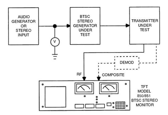
Figure 4-4: Example of Equipment Interconnections
