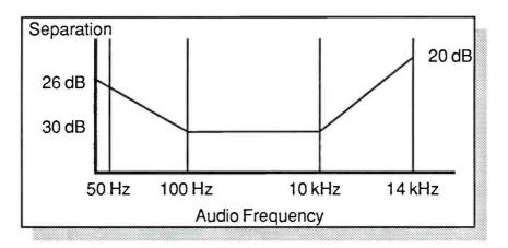
Figure 2-3: Minimum Stereo Requirement with Encoding of L-R
