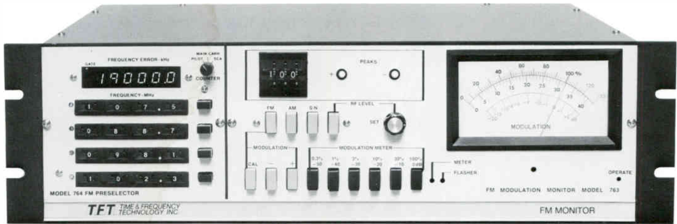
Model 763 FM Modulation Monitor with Model 764 tuneable RF Preselector option
