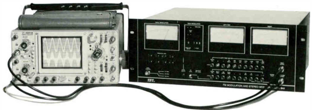
Figure 3: Model 844 permits front panel waveform monitoring.
