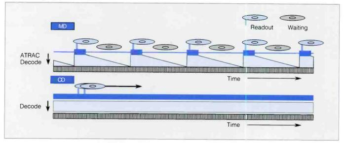
Fig. 3 Interval Reading During Shock or Movement
