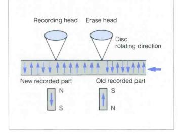
Fig. 19 Data Rewriting with Two Lasers in One Rotation
