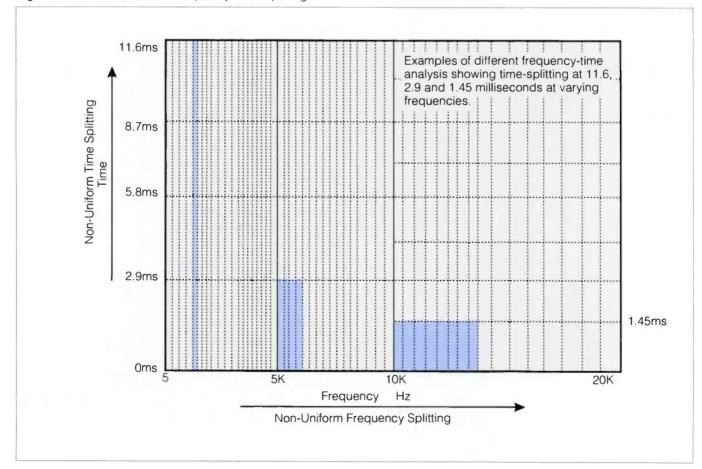
Fig. 17 ATRAC Non-Uniform Frequency-Time Splitting
