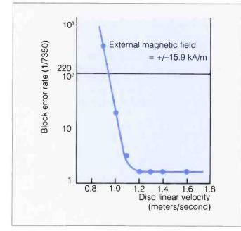
Fig. 22 Block Error Rate with Magnetic Field Modulation
