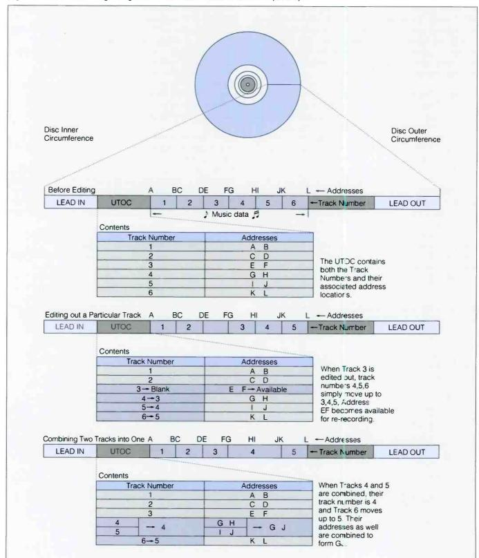
Fig. 5 Track Re-numbering Using the MiniDisc User Table of Contents (UTOC)
