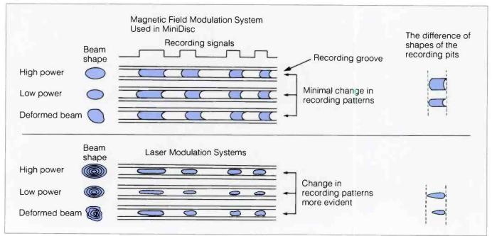
modulation, the latter half will become thicker, as shown in Fig. 23, creating a shape like a tear drop. This is because heat from the laser easily accumulates in the latter half. Shapes like this result in increased jitter upon playback. This problem, however, can be solved by pulsed laser output.
