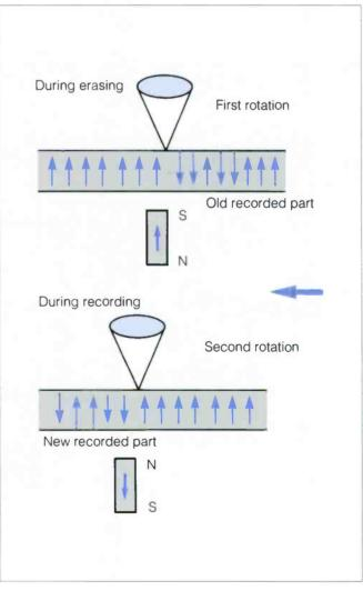
2. A single laser is used for these two tasks, with old data erased in the first rotation, and new data recorded in its place on a second rotation. (Fig. 20)
