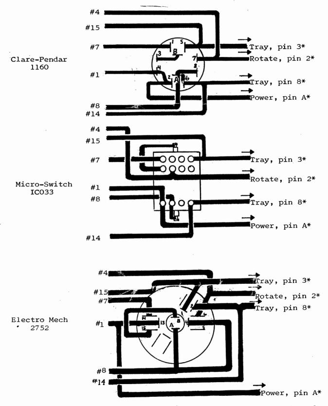
(\*)Wires leading to other switches are in reference to only Clare- Pendar pin numbers. If other switch is also a replacement, consult corresponding drawing.
