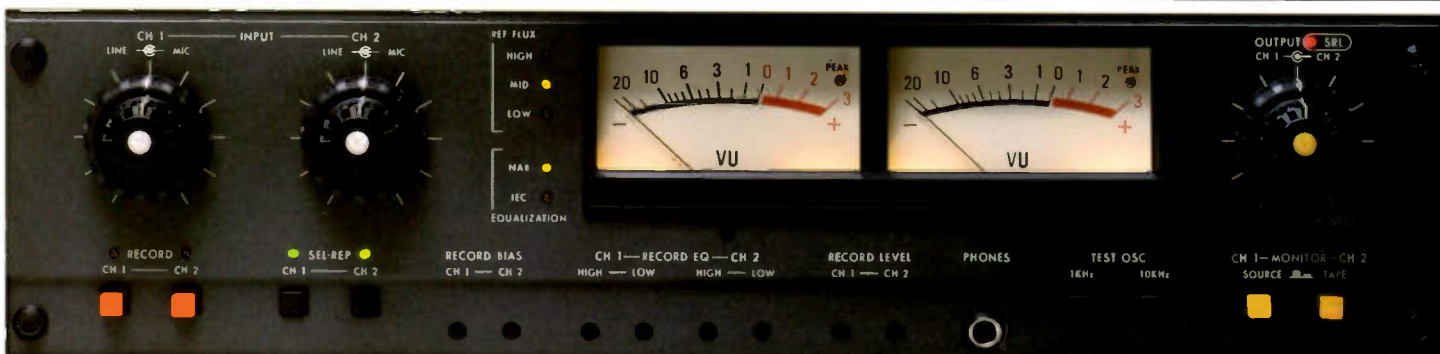
Electronics control panel features access to electronics adjustments for Record Bias, High & Low-speed Record Equalization, and Record Level. A dual frequency test oscillator is built-in.
