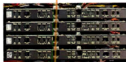
Easy access electronics with plug-in circuit boards put all adjustments for each channel on a single card.
