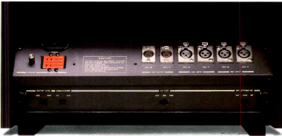
Rear panel features professional XLR-type connectors for all inputs and outputs, switchable output level (+4 dBm or -10 dBV); selectable equalization (IEC/NAB); selectable record fluxivity level calibrations (185, 250 & 320 nWb/m); microphone attenuator (20 dB pad) and the remote transport control jack.
