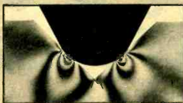
Elliptical stylus at 2 grams.
