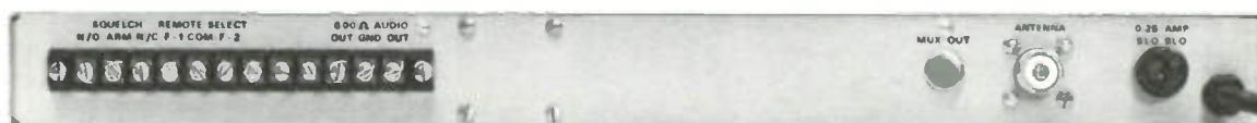
Rear view of Receiver. Barrier strip provides for remote selection of operating frequencies and audio output.
