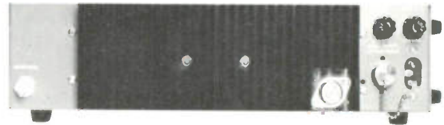
Rear view of Transmitter. Separate fuses and input connectors are provided for AC and DC operation. Note protective cap on DC input. RF output is shown at left.
