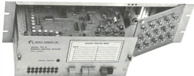
Front View, Transmitter Unit, showing full access. Note LED channel indicators in lower-left of front panel.
