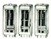
These high grade two band coils are compactly and efficiently designed to provide a type of coil well suited for marine receivers and for general ex-perimental and custom set builders. Broadcast band windings are duo-lateral wound and short-wave windings are solenoid wound. High frequency trimmer condensers for each band are a part of the coil assembly and are adjustable from
