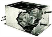
Miller industrial filters are designed for all types of radio interference producing devices and are highly effective at broadcast and short wave frequencies. The unique filter circuit, consisting of two duo-lat-eral wound chokes and two single layer solenoid chokes combined with two 2. mfd. non-inductive wound paper dielectric condensers.
