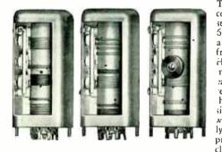
Three band all-wave coils similar in construction to our Series 528 and for use with a 455 KC intermediate frequency amplifier. High frequency trimners are provided for each band and are acressible for adjustment hrough holes in the side of the shield. All windings are thoroughly impregnated for protection under all climatic conditions.
