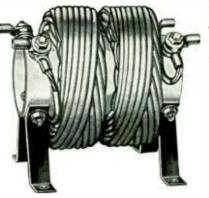
Miller Heavy Duty Line Filter Chokes are wound on electrical porcelain forms measuring 4" in diameter by 8" long. All windings are of the duolateral type and use double cotton covered stranded cable expressly made for this purpose. Copper terminal lugs and brass bolts are used on all current-carrying parts. Four sturdy steel mounting brackets are provided with each choke. Windings are thoroughly impregnated with glyptal varnish and baked. In
