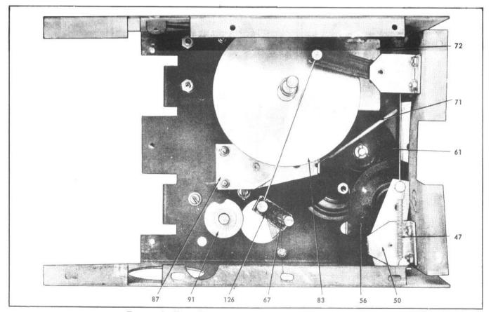
Figure 4. Tape Transport with Front Panel Removed.
