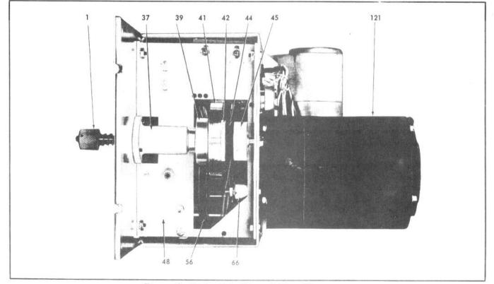
Figure 2. Right Side View of Tape Transport.
