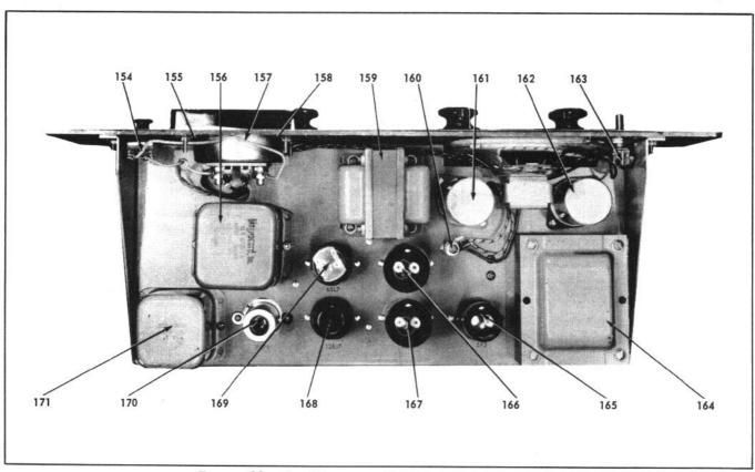
Figure 12. Top View of PT6-6J Amplifier Chassis.
