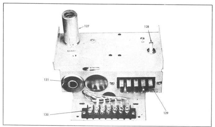
Figure 8. Top View of Bias Oscillator Chassis.
