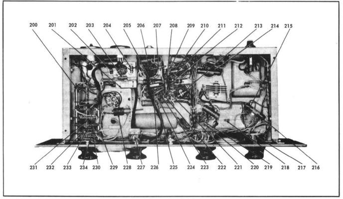
Figure 11. Bottom View of PT6-6J Amplifier Chassis.
