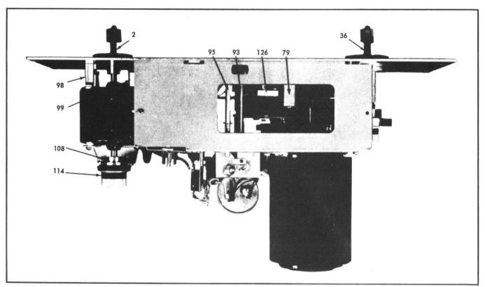
Figure 3. Bottom View of Tape Transport.
