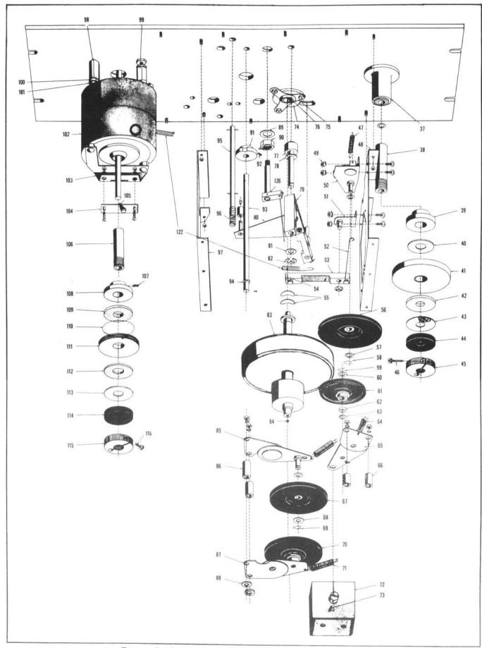
Figure 6. Exploded View of Parts Below Front Panel.
