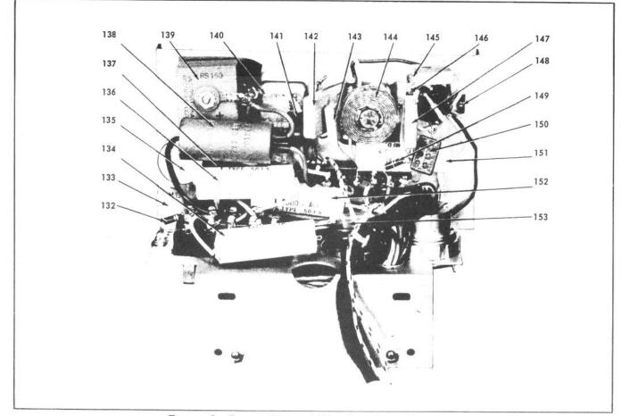
Figure 9. Bottom View of Bias Oscillator Chassis.
