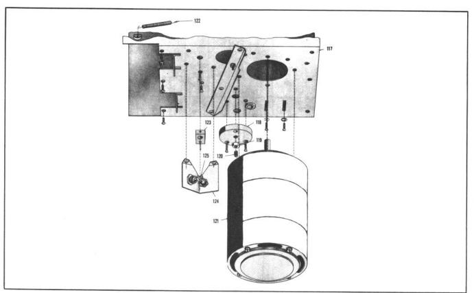
Figure 7. Exploded View of Parts Below Rear Panel.
