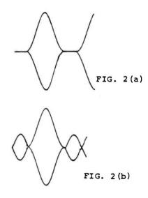
FIG. 2 TWO TYPES OF OVERMODULATION
