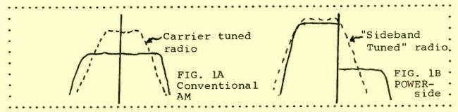
FIG. 1 illustrating enhancement of the lower sideband.
