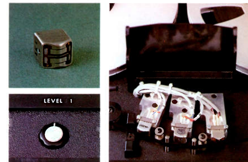
The flip-up cover exposes tape for easy editing.
