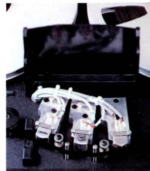
The flip-up cover exposes tape for easy editing.
