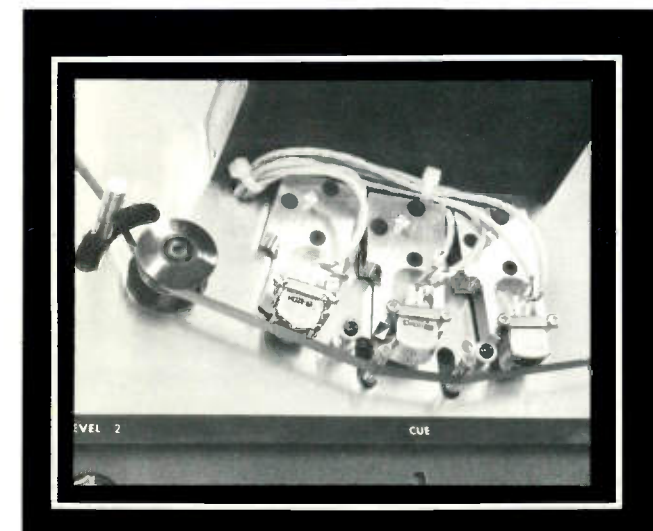
Flip-top head cover for editing accessibility. Excellent phase stability — the five tape guides are secured directly to the deck plate, assuring a fixed and accurate tape travel path for precise phase alignment.
