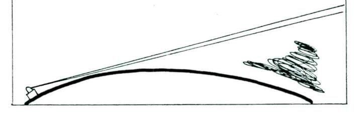
The storm cell and the leading edge of low altitude clouds are within view of the radar. However, the cell following the first one can not be seen because it is not tall enough. The dash lines indicate the radar beam when it is tilted to find the top of the cell.
