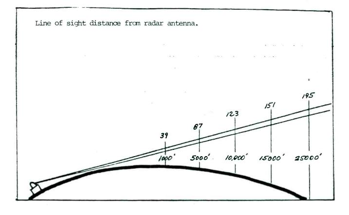
"Ducting" or SUPER REFRACTION of radar beam. Temperature Inversion
