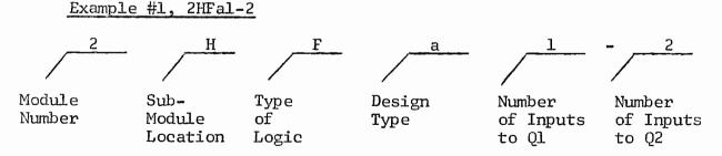
Thus 2HFa2 refers to a submodule located in position H of module 2. This submodule is a binary (flip-flop) of the "a" circuit design and has a "set one" input as well as the standard count inputs. Figure 16 provides all information on this submodule type; schematic diagram component layout and Bill of Material. Figure 19 shows submodule location and pin numbers on the harness board.
