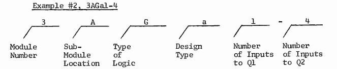
Thus 3AGal-4 refers to a submodule located in position A of Module3. This submodule is a double gate of the "a" circuit design. One input resistor is provided for the gate whose output is submodule pin 12. Four input resistors are provided for the gate whose output is submodule pin 17. Figure 17 provides all information on this submodule type; schematic diagram, component layout, and bill of material. Refer to Figure 19 for submodule locations and pin numbers.
