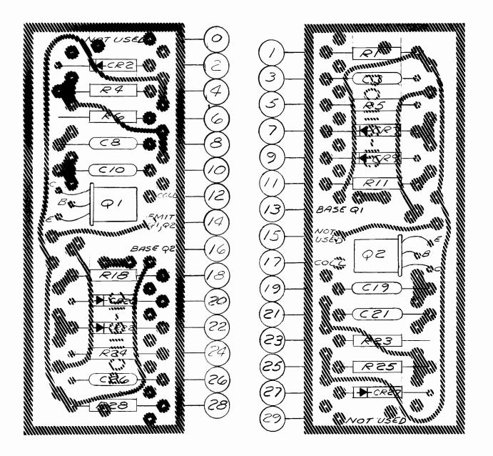
NOTESS I-FOR EXPLANTION OF DESIGN VALUES SEE APPENDIX I. 2-RESISTORS RE9 AND R30 ARE NOT NORMALLY USED. SEE CHART OF SUBMODULES OR PARTS LIST FOR LISTING OF SUBMODULES WHICH USE THESE RESISTORS.
