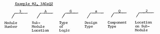
Thus 3AGaQ2 refers to a transistor located in mounting clip number two of submodule A in module number 2. Referring to the Double Gate submodule reference drawing figure 17A shows that the transistor is used in the second gate and for the "a" design is a 2N404.
