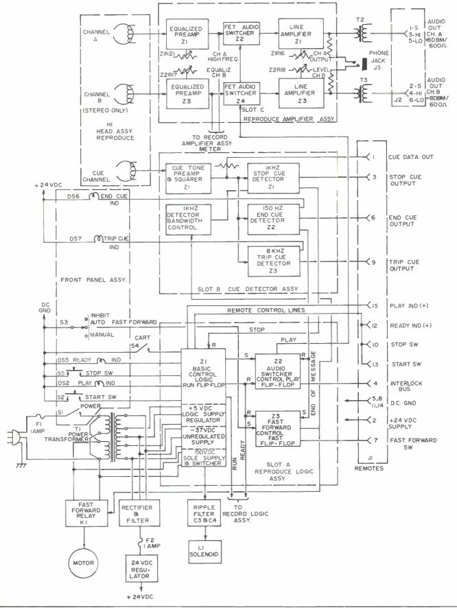
FIG. 6. Block Diagram Reproduce Electronics
