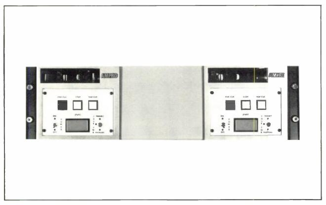
FIG. 13. Rack Mount with Fill Panel
