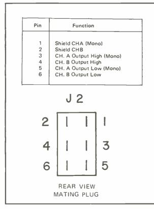
FIG. 15 Audio Output Connection Table J2
