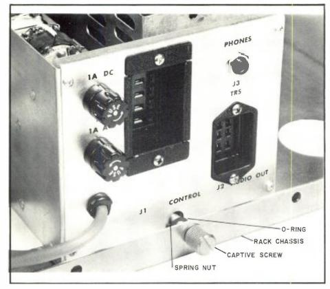
FIG. 12. Rack Mount Detail, Rear View
