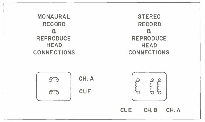
FIG. 24. Head Connections
