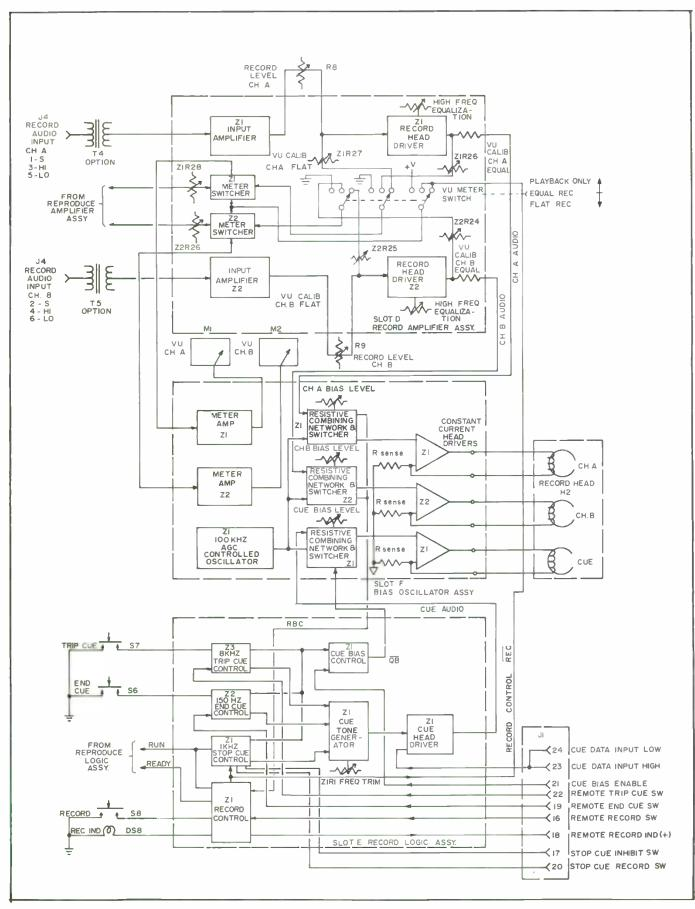
FIG. 7. Block Diagram Record Electronics
