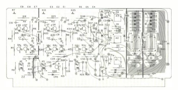
FIG. 46. Bias Oscillator P.C. Board Layout
