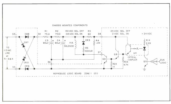
FIG. 10. Simplified Schematic-Solenoid Supply & Control Circuit
