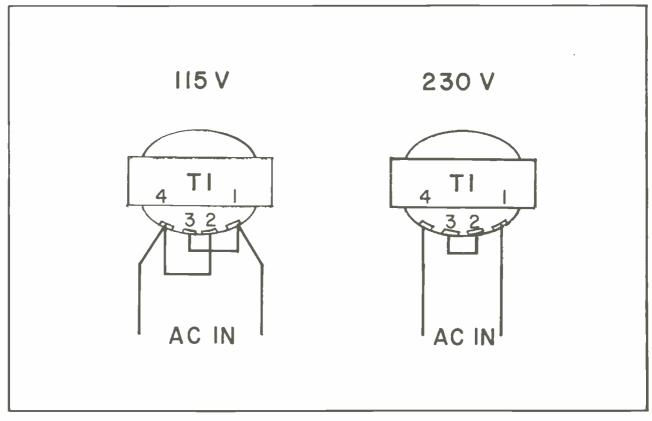
FIG. 14. Power Transformer 115/230 VAC Connections
