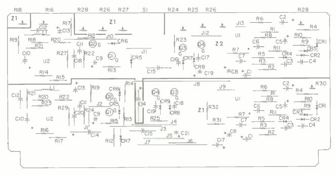
FIG. 44. Record Amplifier P.C. Board Layout
