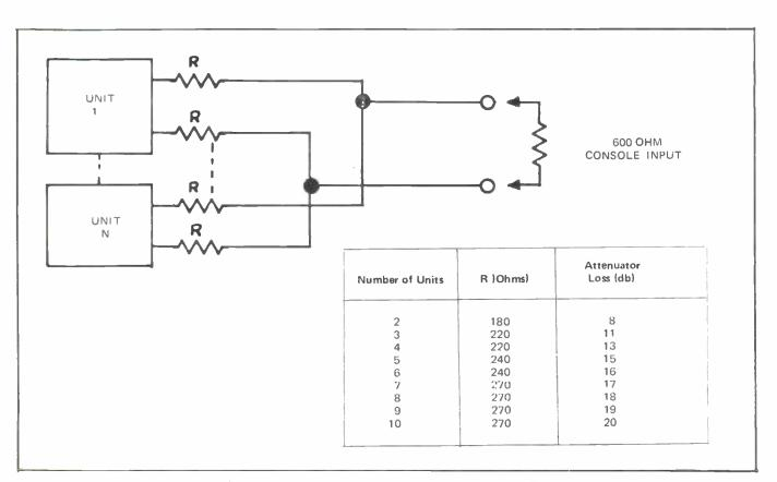
FIG. 18. Constant Impedance Combining Network Table
