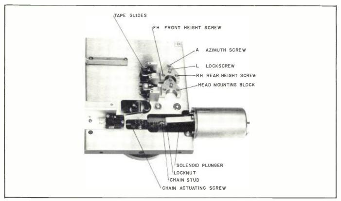
FIG. 21. Solenoid Pressure Adjustment
