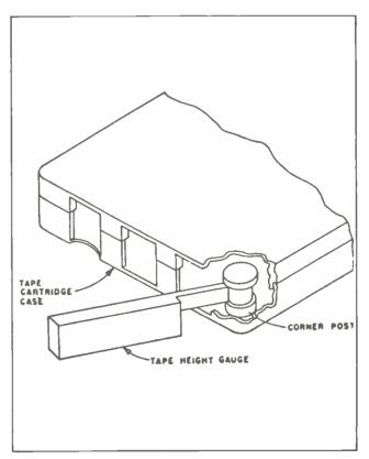
FIG. 26. Corner Post Adjustment
