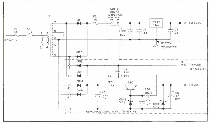
FIG. 9. Simplified Schematic Power Supply Circuit
