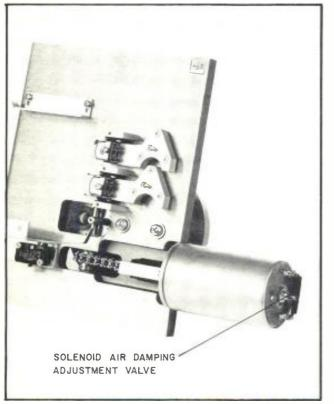
FIG. 22. Solenoid Damping Adjustment
