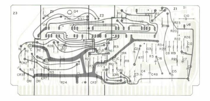
FIG. 38. Record Logic P.C. Board Layout
