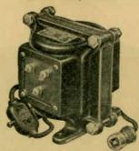
The BH-1 Transformer is especially designed to supply filament and plate voltage for the UX 171 or UX 210 type tubes. This transformer has two secondary plate voltages, high enough to give a D.C. output of 180 volts for the UX 171 tube and 400 volts for UX 210 tubes. This transformer has a separate filament winding for the rectifying tube and another for the amplifying tube. Type BH-1 Transformer, 110
