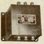
The Acme Tone Filter contains an impedance of the proper value through which the plate of the power tube is supplied, and which will carry enough current continuously without heating or deterioration. Also cased in the tone filter is a 4 mfd. through which the A. C. component of the power tube passes to the speaker.
