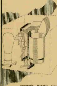
Automatic Variable Coup-ling—same control operates tuning condenser and prim-ary coil coupling simultan-eously, gives maximum and equal amplification and selec-tivity over entire tuning range.
