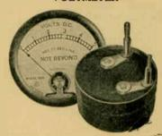
A high resistance voltmeter (25 ohms per volt) is specified because one not of high resistance consumes enough current for operation to cause a serious drain on the batteries and rob the tubes of current required for their proper performance.
