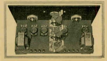
It is a known fact that a vacuum tube has a natural tendency to oscillate at the lower wave lengths. In the Ultimax receiver practically uniform selectivity is obtained on low and high wave lengths alike, due to Ultimax Unit. This Unit is inserted in the plate circuit and superimposes a current on the oscillations of the tube.
