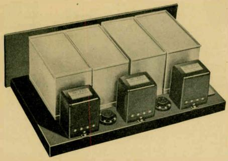
The Silver Shielded Six is one of the highest types of broadcast receivers ever developed, and is the result of painstaking engineering work over a period of years. The circuit employed consists of three stages of tuned radio frequency amplification, a detector and two stages of audio amplification.
