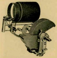
Here is the tuning unit the radio world has been waiting for—a harmonious assembly of coil, condenser and shield providing automatic, grad-uated coupling of the primary coil throughout the range of condenser settings.
