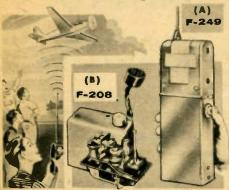
(A) RADIO CONTROL TRANSMITTER: Assembled-tested-guaranteed. No license examination required for operation. Crystal controlled for stability and to meet F.C.C. regulations. Uses powerful 3A5 tube for range of approximately one mile. Will operate any 27.255 mc R/C receiver. Overall dimensions only 8½" x 2¾" x 1¾" – just a handful! Includes antenna – tube – crystal – and instructions. Less Batteries. Shpg. wt., 2½ lbs.
