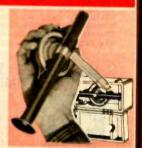
Designed for the small boat owner—fisherman—hunter—camper. A combination of an "alidade" type sighting tube and a jeweled pivot, liquid compass, Takes instant, accurate sightings on land-marks and converts them into compass bearing. Fixes your position automatically—easily. Graduated in increments of 1° with each 10°s called out. Constructed of heavy brass throughout, antimagnetic & corrosion-proof. Complete with instructions. Imported. Shpg. wt., 3 ibs.
