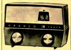
Provides superb high fidelity FM Reception by just plugging into any amplifier and speaker, phonograph, T. V., Custom Music System, or tape recorder. Super selective reception even in fringe areas. Exclusive no drift cooxial tuner and associated circuitry reduce operation to just 2 knobs. Built in antenno. 6 tubes. Modern style cabinet. Size 61/4" Wide. 4" Deep. 41/4" High. Shpg. wt., 4 lbs.
