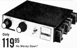
SPECIFICATIONS: Frequency Coverage: 20-54 MHz, Plate Power Input: 50 Watts (100 Watts PEP). Minimum RF Orive: 1/2 Watt. Maximum RF Drive: 10 Watts. Input Impedance: 50 Ohms, Output Impedance: 40-600 Ohms (50 Ohms Nominal). Amplification Modes: AM, FM, SSB, OSB, CW, Power Requirement: 12 Volts DC (Neg. Ground only). DC Power Cansumption: 27-watts idling, 120-watts at full input.
