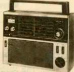
FREQUENCY RANGE: FM 87.5-108 MHz SW2 3.5-7 MHz AM 530-1,605 kHz SW3 7-14 MHz SW1 1.6-3.5 MHz SW4 14-26.1 MHz
