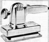
Heavy-duty electric sander with \( \frac{\pi}{n} \) orbital or straight line stroke. Features 2.0 amp, universal series wound motor. Heavy-duty ball bearing and self-lubricating sleeve bearings. Pad size: \( \frac{3\pi}{n} \times \frac{3\pi}{ 13 H 71020 Shpg. wt., 51/2 lbs.
