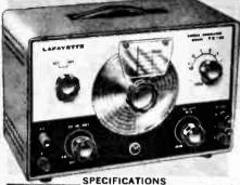
Full frequency range: 6 Fundamental bands—120-320 kHz 320-1000 kHz 1-3.5 MHz. 3.2-11 MHz 11-38 MHz 36-130 MHz; 1 harmonic band 120-260 MHz. Frequency Accuracy: ±2%, Audio Output: to 8 v., (Vernier tuned) High-Low RF out-put Terminals.
