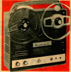
Noise Ratio: Better than 42 db; Bias and Erase Frequency: 60 kHz; 2 inputs: Microphone and Auxiliary; 1 output: External speaker. For 110-120 v., 50/60 Hz AC. Housed in solid vinyl case with built-in accessory compartment and carrying handle. Size: 11% x 12¼ x 6½°D. Imported. Shog. wt. 16 lbs.
