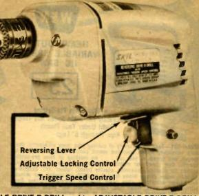
1/4" ADJUSTABLE DRIVE-R-DRILL Model 596-5 rated at 2.5 amps, 0-2000 rpm Forward/Reverse. Capacity 1/4" in steel, 1/2" in wood. Shpg. wt., 4 lbs. 13 R 6931 Net 29.88
