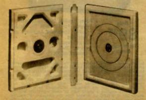
Lafayette "Poly-Planar" wafer-type component loudspeakers employ a lightweight acoustic panel supported by a frame of polystyrene plastic material to reproduce a range of frequencies from 40 cps to 20,000 cps. This material also permits the speakers to be made impervious to extremes of temperature, humidity, shock, and vibration. There is also a minimum of piston-motion resulting in low distortion and high electromagnetic efficiency.
