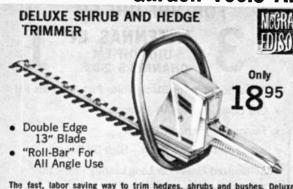
The fast, labor saving way to trim hedges, shrubs and bushes. Deluxe "Roll-Bar" handle allows maximum comfort and safety—adjusts for any angle cut. 2-cutting edges, each with 16-teeth—cuts 12" swath in either direction. 13" blade cuts at 1850 strokes per minute. Die-cast aluminum housing with bright finish and enamel finish roll-bar. Fingertip On/Off switch. Hardened spring steel teeth are self-sharpening. 2.6 amp, 115 volt, 50/60 cycle AC motor. Shpg. wt., 6 lbs.
