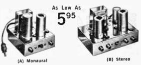
(A) Self Powered Monaural Preamplifier. For use with any Hi-Fi amplifier that does not have low level inputs for magnetic cartridges, tape heads, or microphones. Response:  $\pm 2$  db at 30-20,000 cps. Gain (phono): 40 db, 5 mv. input for 1 volt output. Output impedance: 100,000 ohms. Features phono tape equalization switch, 2 input jacks, 16 inch output lead with plug. For 105 125 volts 50-60 cps 4 watts AC. Size: 334x354x3134x. Less 12AX7 Tube. Imported. Shpg. wt., 232 lbs.
