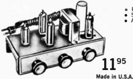
Push-Pull Audio Output Stage-Inverse Feedback Circuit
