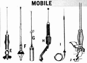
(E) FAMOUS LAFAYETTE ALL STAINLESS STEEL CB MOBILE ANTENNA Full quarter wave 102-inch stainless steel whip, heavy-duty chrome plated stainless steel spring and swivel ball jointed base designed for mounting on any surface. Base has lug terminals for 42 - 7002 cable assembly. Perfect for rear deck mobile mounting.
