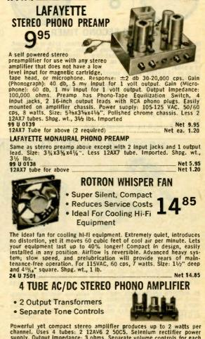
Powerful yet compact stereo amplifier produces up to 2 watts per channel. Uses 4 tubes: 2 12AV6 2 50C5. Selenium rectifier power supply. Output Impedance: 3 ohms. Separate volume controls for each channel. Size: 6<sup>1</sup>/<sub>4</sub>x2%,x4<sup>4</sup>. Less tubes. Imported. Shpg. wt., 3 lbs. 99 U 0154 36 U 9002 Kit of 4 tubes \_\_ Net 2.60
