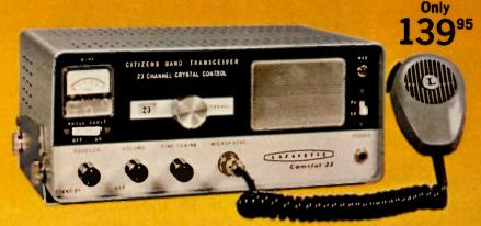
• 15 Tube Performance with 10 Tubes, 2 Transistors and 9 Diodes **Crystal Frequency Synthesizer**
