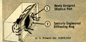
The loudspeaker is mounted on a baffle recessed in the cabinet shell with the front-plate extending partially across the front surface of the baffle forming ducts or tubes from the port openings to the
