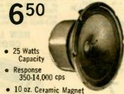
Capable of reproducing virtually undistorted sound from 350 to 14,000 cps, the recommended crossover frequencies are at 350 cps and 5,000 cps. Power handling capacity: 25 watts. Cone Resonance: 150 cps. Impedance: 8 ohms. 10 oz. ceramic magnet. Voice coil diameter: 1". Plated steel frame finished in brown baked enamel. Has 4-way binding posts. Shpg. wt., 4½ lbs.
