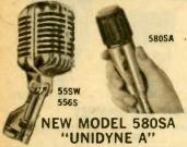
Slim, low cost cardioid dynamic. Ideal for controlling feedback in P.A. systems and improving home recording. Features rugged dynamic element with true cardioid unidirectional pickup pattern, built-in On-Off swtch and 15-foot attached shielded cable. High impedance. Response: 50 to 11,000 cps. Output, -58 db. Satin chrome case with "Armo-Dur" cap and stainless steel mesh grille, 6\%"x1\%". Shpg. wt 2 lbs.
