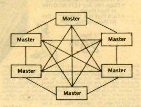
All-Master Intercom System incorporates up to six separate master stations enabling 3 private conversations or a 6-station conference to be held. Utilizes a three-position switch for listening, momentary talking, or dictating; and a five-station selector-call switch.
