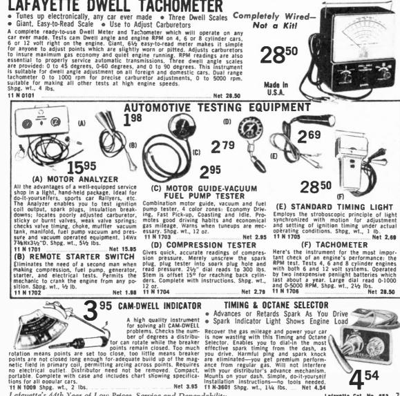
ber of degrees a distributor can rotate while the breaker points remain closed. Too much rotation means points are set too close, too iittle means breaker
