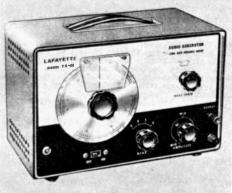
FACTORY CALIBRATED AND TESTED . LOW DISTORTION . FREQUENCY RANGE - SINE WAVE: 20 Cps-200 KC IN 4 BANDS, SQUARE WAVE 20-25 KC FREQUENCY RESPONSE ±1.5DB, 60CPS - 150KC 41/2" VERNIER DIAL
