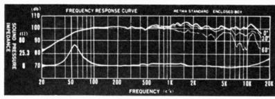
= 20 TO 20,000 CPS (40 TO 16,000 CPS  $\pm$  3 DB) = HIGH EFFICIENCY = HIGH EXCURSION WOOFER WITH UNIQUE "CONICAL STIFFENER" = HANDLES HEAVY BASS PASSAGES WITHOUT "DOUBLING"
