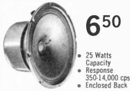
Capable of reproducing virtually undistorted capable of reproducing virtually undistorted sound from 350 to 14,000 cps, the recom-mended crossover frequencies are at 350 cps and 5,000 cps. Power handling capacity: 25 watts. Cone Resonance: 150 cps. Im-pedance: 8 ohms. 10 oz. ceramic magnet. Voice coil diameter: 1". Plated steel frame finished in brown baked enamel. Has 4-way binding notes the wet 416 the binding posts. Shpg. wt., 41/2 lbs. Net 6.50 21 N 4718
