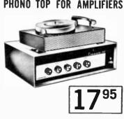
4-speed (16, 33<sup>1</sup>/3, 45 and 78 RPM) phono-graph turntable is designed to fit on top of the amplifier and is easily mounted with 2 thumb screws. Takes records up to 12". High quality ceramic pickup-turnover type with dual synthetic sapphire stylus. Power re-quirements: 15 waits, 117 volts, 60 cps. Durable finish. Size 12x9<sup>1</sup>/4x4<sup>1</sup>/2". Shpg. wt., 8 lbc 8 lbs.
