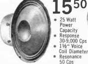
Ideal for assembling 2- and 3-way speaker systems at a budget price. Enclosed magnet structure – completelly dust-proof. Compli-ance of outer cone and inner spider carefully calculated for best bass response. 114 lb. ceramic magnet, 8 ohm impedance. Has 4-Way binding posts. Cone Resonance 50 cycles. Shpg. wt., 8 lbs. 21 N 4716 Net 15.50
